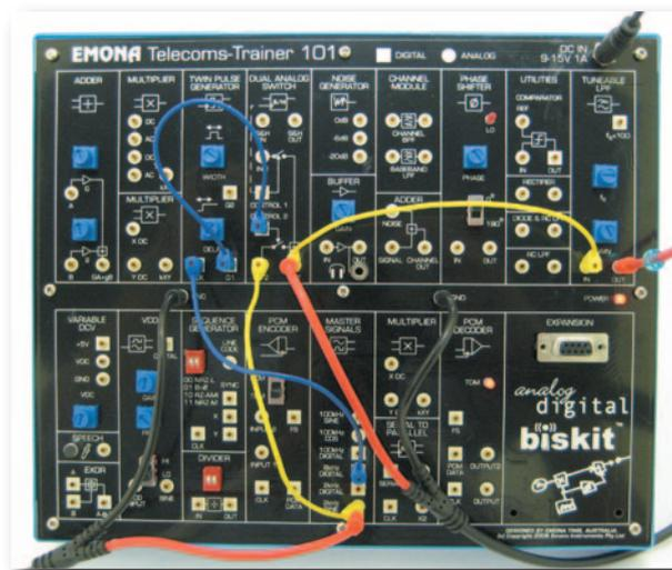
Patching a sampling & reconstruction experiment uses 4 of the ETT-101's functional blocks:
