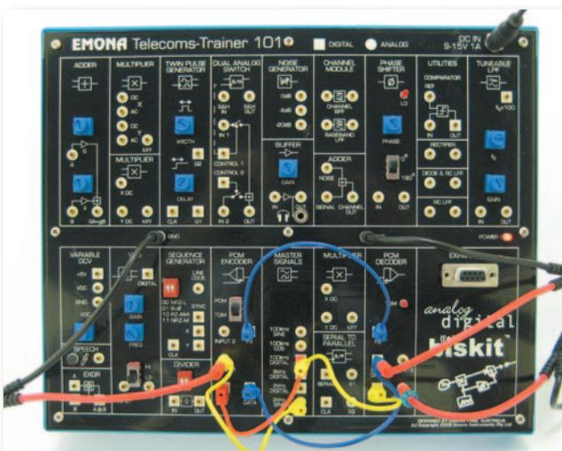
Patching a PCM encoding & decoding experiment uses 3 of the ETT-101's functional blocks:
