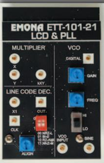
The ETT-101-21 Line-Coding & PLL Experiments expansion board for implementing Line-Code Decoding, DPSK demodulation, and FM PLL demodulation experiments.
