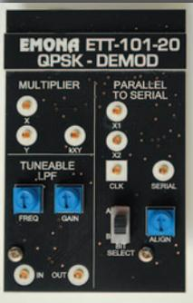
The ETT-101-20 QPSK Experiment expansion board will allow a complete QPSK modulation / QPSK IQ-branch demodulation experiment to be implemented.
