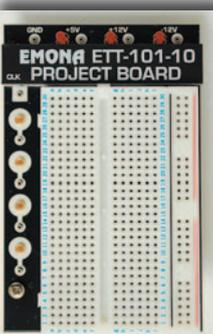
The ETT-101-10 Electronic Circuits Project Experiment board allows students to build their own analog and digital electronic circuits and interface them with the ETT-101 functional blocks. Example circuits include passive and active filters and oscillators.
