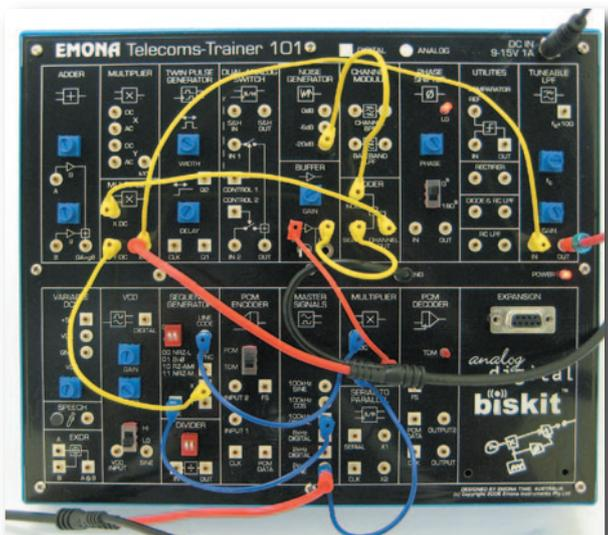
Patching an DSSS modulation and demodulation in a noisy channel experiment uses 8 of the ETT-101's functional blocks:
