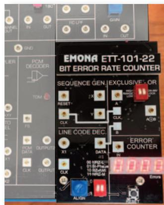
The ETT-101-22 BIT ERROR RATE COUNTER EXPERIMENTS BOARD includes four individual modules for implementing fundamental Bit Error Rate counting instrumentation.
