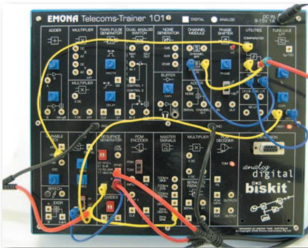
Patching an FSK modulation and demodulation experiment uses 7 of the ETT-101's functional blocks:
