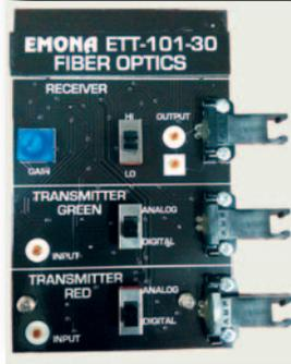
The ETT-101-30 FIBER OPTICS Experiment expansion board includes three independent functional blocks, providing an electrical-optical and optical-electrical interface for the ETT-101. When added to the ETT-101 it will allow a complete optical link to be established, for analog or digital signals.
