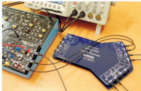
The ETT-101-31 FIBER OPTIC COUPLERS and WDM FILTERS Experiment expansion board includes four independent functional blocks. When added to the ETT-101 and ETT-101-31 it will allow a complete bi-directional and WDM fiber optic links to be implemented.
