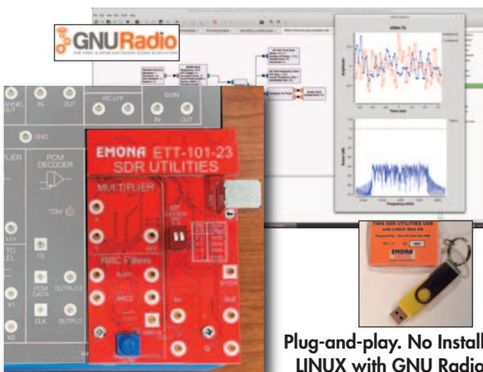
The ETT-101-23 SOFTWARE DEFINED RADIO BOARD is supplied as a complete, zero install solution. One step boot-and-run USB thumb drive has pre-installed LINUX with the full GNU Radio.
